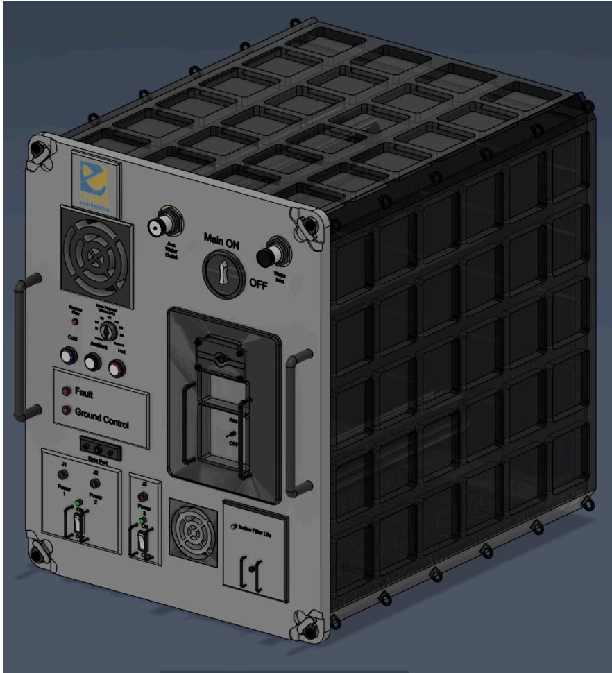
Figure 6: CAD Model of the EBPWD Housing with Interface Panel.
