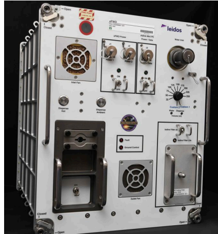
Figure 2: Leidos Exploration Potable Water Dispenser (xPWD) 22 .
