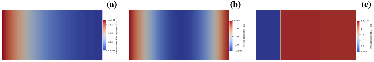
Figure 12: P2D-Based Model t = 27s ( 75 \mu\text{m} Cathode, 5 \cdot 10^{-2} \text{ A/cm}^2 Case) (a) \text{Li}^+ Concentration, (b) Potential In Electrolyte, (c) Potential In Solid Phase
