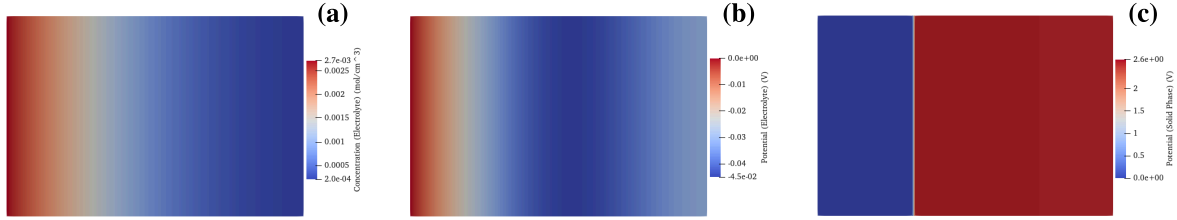
Figure 4: P2D-Based Model t = 3600s ( 50 \mu\text{m} Cathode, 4 \cdot 10^{-2} \text{ A/cm}^2 Case) (a) \text{Li}^+ Concentration, (b) Potential In Electrolyte, (c) Potential In Solid Phase
