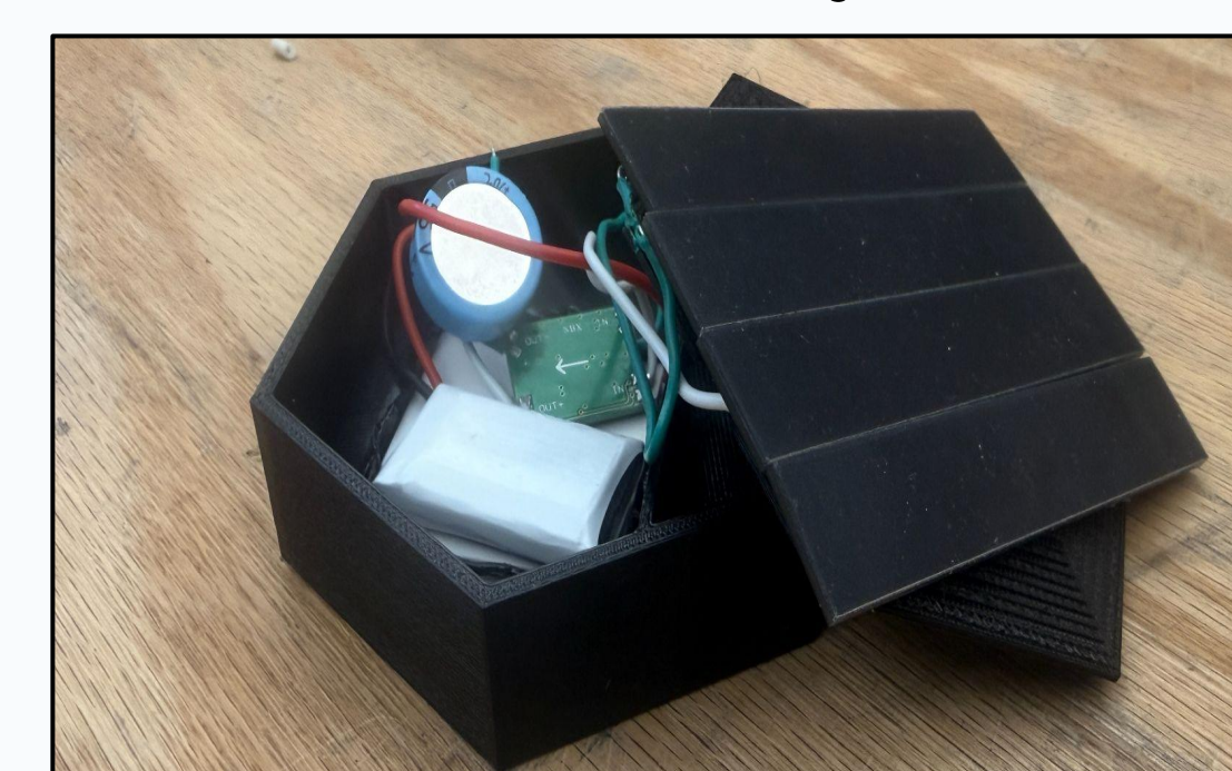
Power harvesting test setup, with photovoltaic cells and thermoelectric generator.
