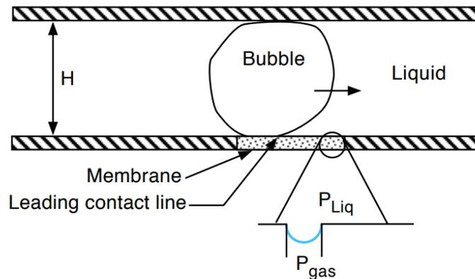
**FIGURE 4: Gas bubble passing by a hydrophobic membrane (Balasubramaniam et al., 2019)**
