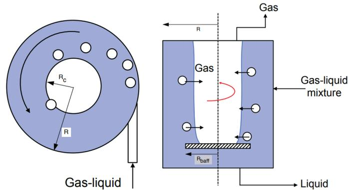
**FIGURE 3: Centrifugal Cyclonic Separation of Entrained Two-Phase Flow (Balasubramaniam et al., 2019)**
