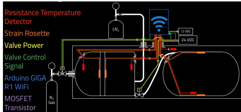
**FIGURE 7: PULSE Control System Wire Routing Diagram**
