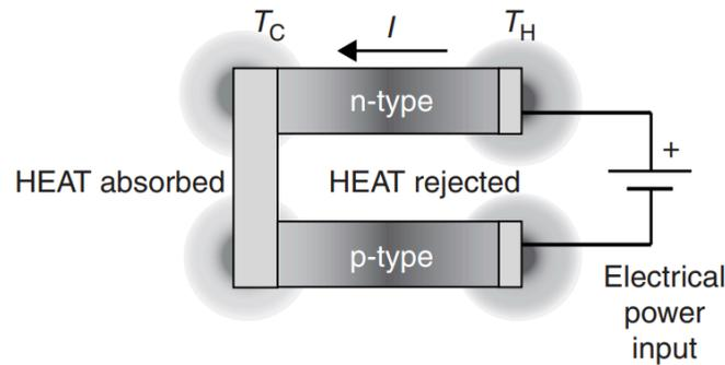
The Peltier effect (Thermoelectric cooling)
