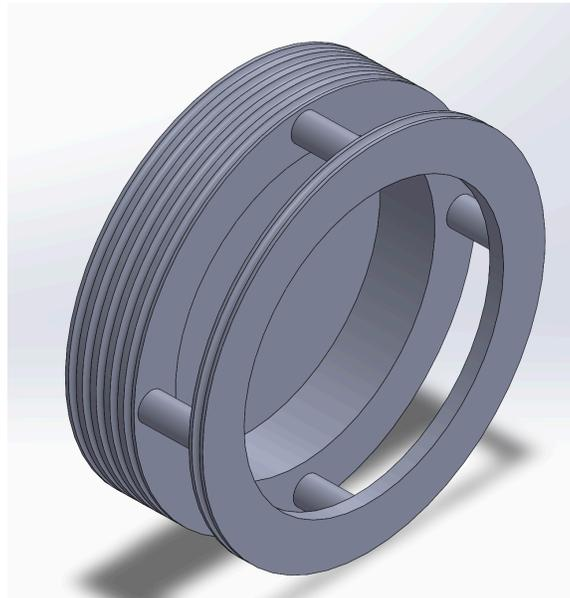
**FIGURE 6: A 3D model of the piston used to expel LN<sub>2</sub>**
