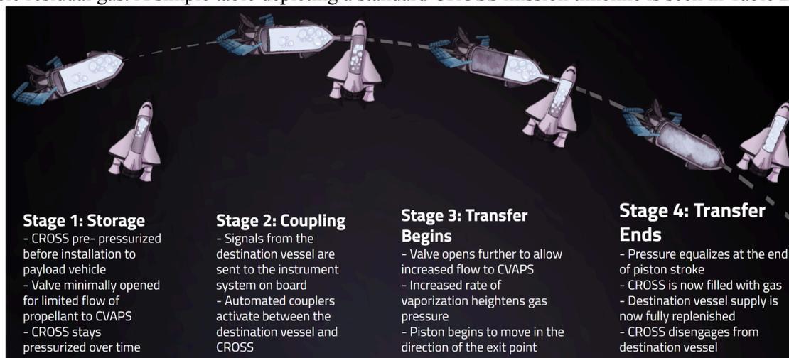
**FIGURE 8: CROSS Concept of Operations**
