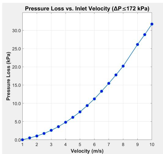
FIGURE 7: Pressure and Velocity Relationship in Transfer Line
