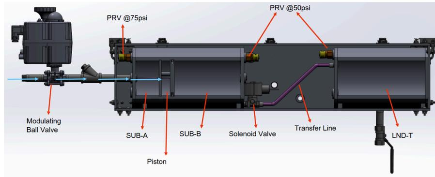
**FIGURE 5: PULSE Apparatus Solidworks Diagram**
