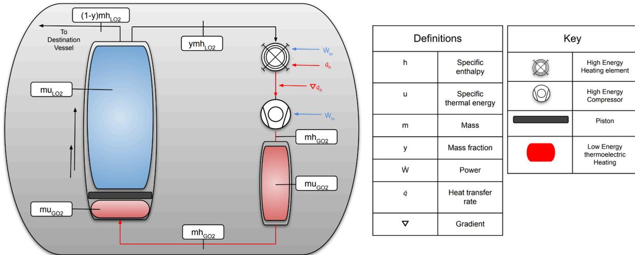
**FIGURE 2: CVAPS Basic Layout Illustrating Major Components and Processes**
