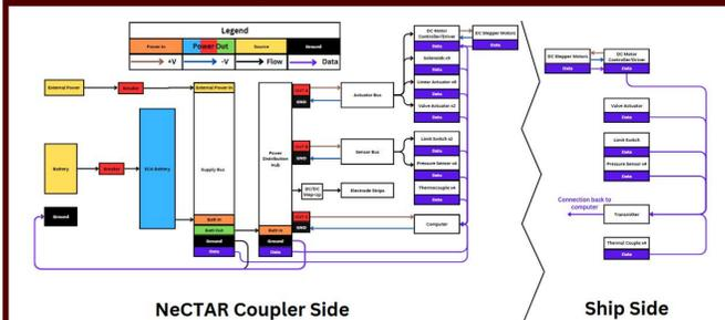
Figure 4. EPS functional block diagram NeCTAR.
