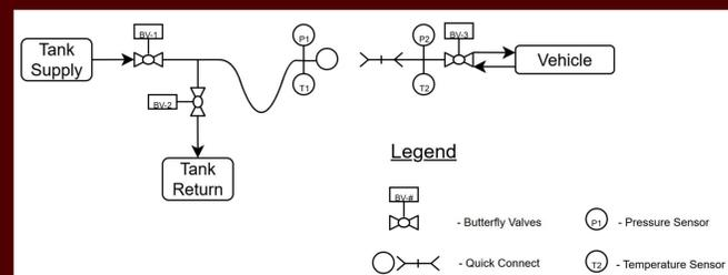
Figure 3. NeCTAR's Piping and Instrumentation Diagram
