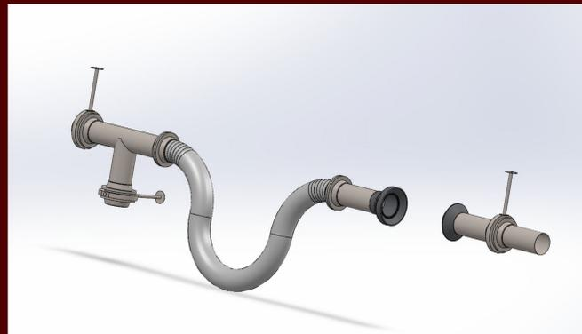
Figure 2. 3D Model of interior NeCTAR pipe-coupler system, to scale.
