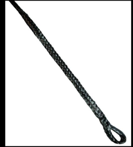
(Left) Tensile Testing Adapter Setup (Right) Dyneema Sample with Brummel eye splice
