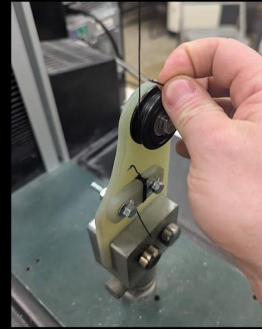
(Left) Tensile Testing Adapter Setup (Right) Dyneema Sample with Brummel eye splice
