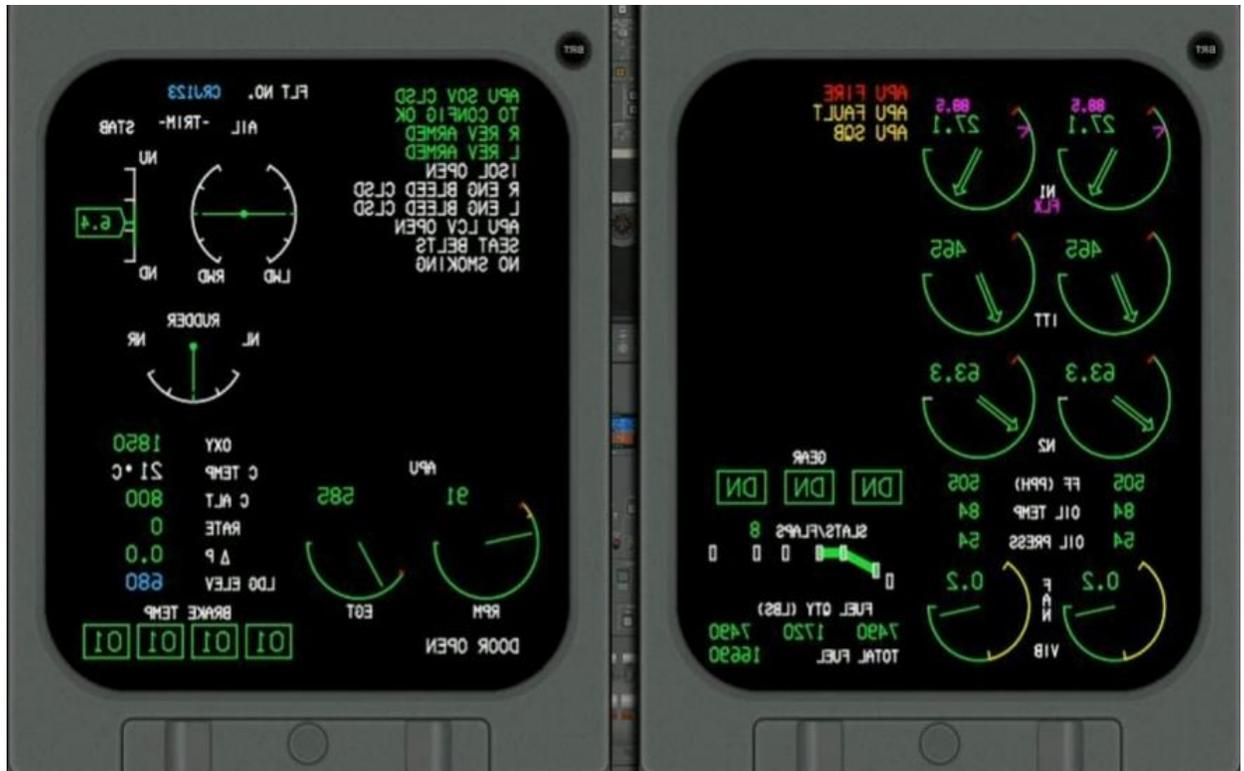
**Figure 2 CRJ-700 EICAS Display (Aerosim Technologies Inc. , 2015)**
