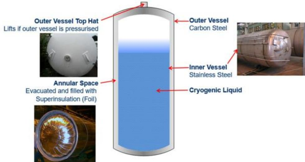
Cryogenic Tanks – typical current construction
