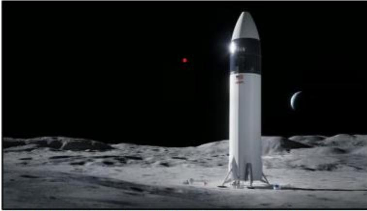
The SpaceX Starship HLS spacecraft, designed for lunar landings, is 52.3 meters tall, 9-meter diameter, and has no heat shield or flaps. It uses landing thrusters, solar panels, and has an elevator system for crew access to the lunar surface.
