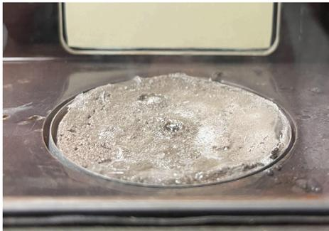
**Fig. 7 Lunar regolith treated with CA.**
