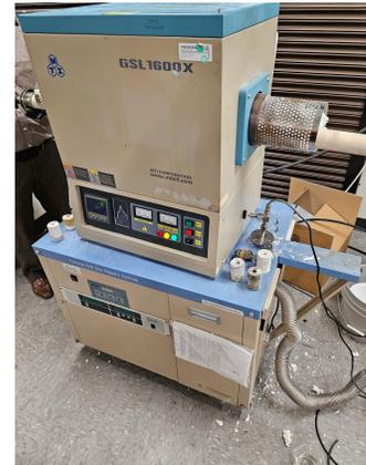
**Fig. 2 Sintering furnace.**
