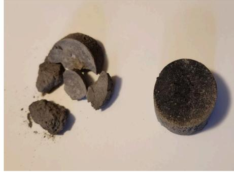
**Fig. 6 Lunar regolith sintered at 1200 °C.**
