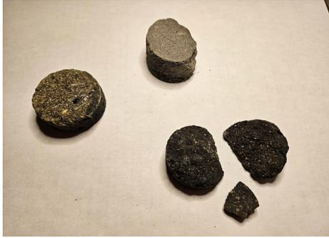
**Fig. 5 Lunar regolith sintered at 1100 °C.**
