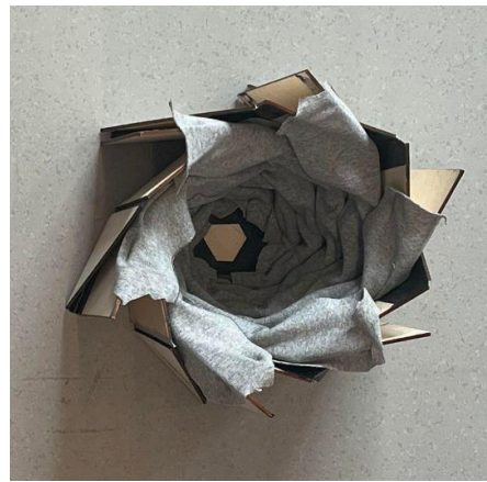
Figure 4: Prototype in its packed configuration. The diameter of this is just over 7 inches.
