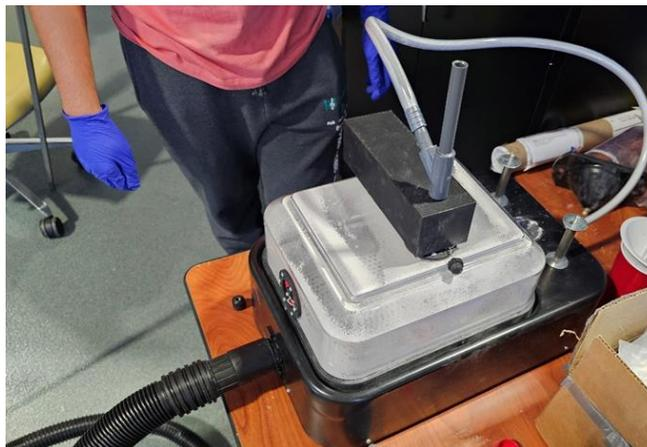
Figure 27: Grit Blaster Experiment Setup
