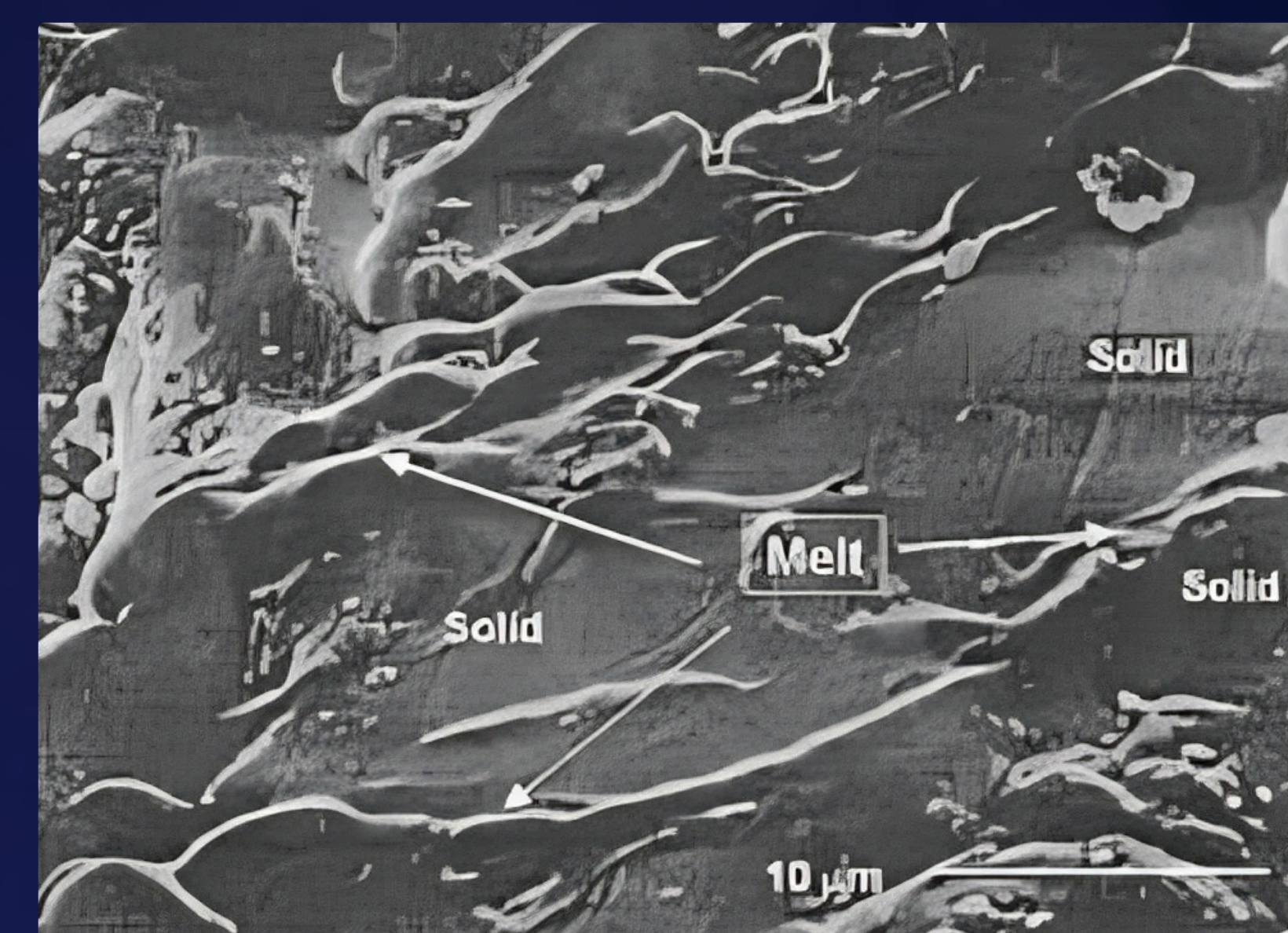
Microwave melting along grain boundaries of mare soil [1]
