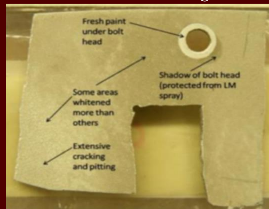
Figure 1. Damage on Surveyor III camera shroud due to PSI. [4]
