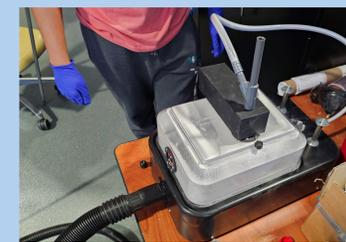
The team modified a grit blaster with simulant feed to evaluate impact and abrasion resistance of WC-Co cold spray coating
