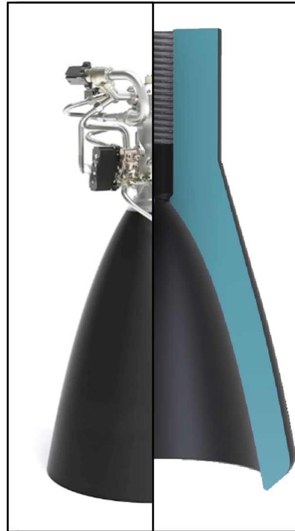
Nozzle Contour Comparison 12:1 scale
