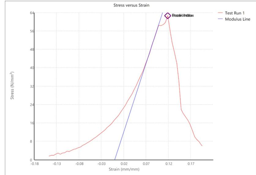
**Figure 9:** Ultimate stress curve for Kevlar, reaching **62.6 MPa**
