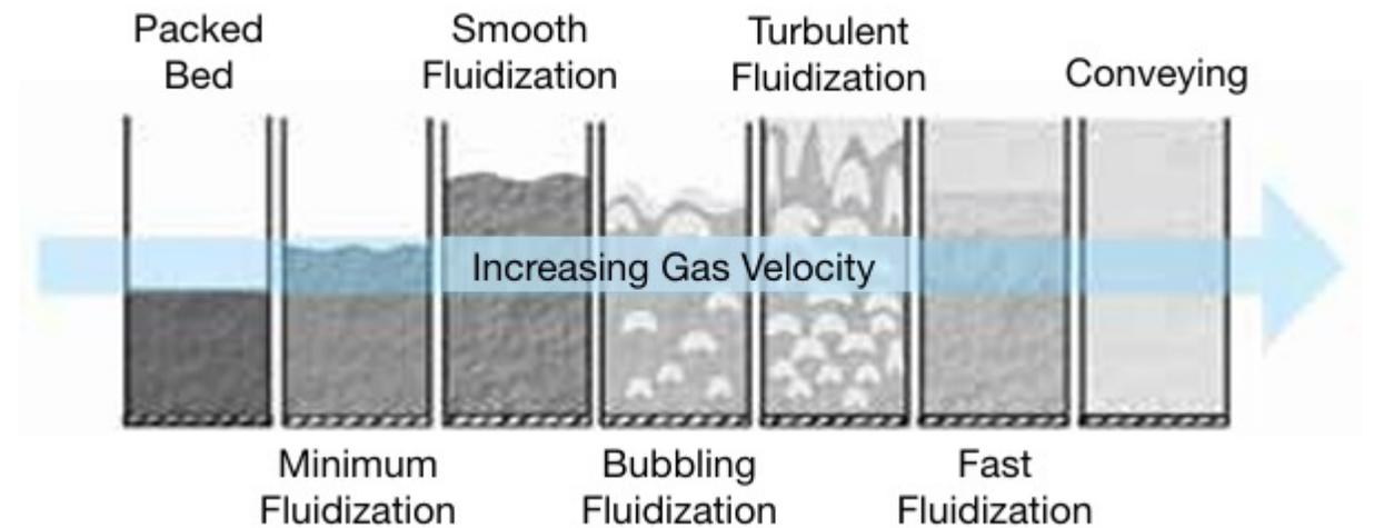
Different types of fluidization (Cocco et al., 2014)
