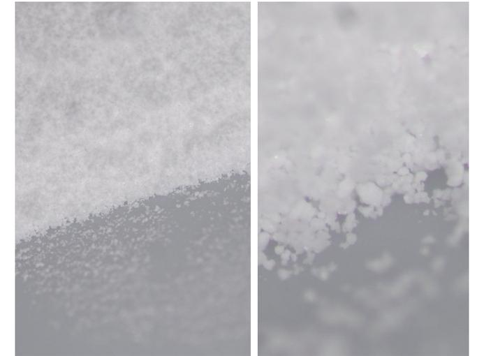
Alumina Powder in Optical Microscope
