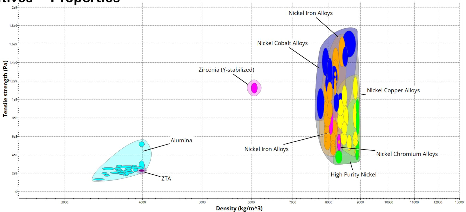
Additives Tensile Strength v. Density Plot (ANSYS® Inc., n.d.)
