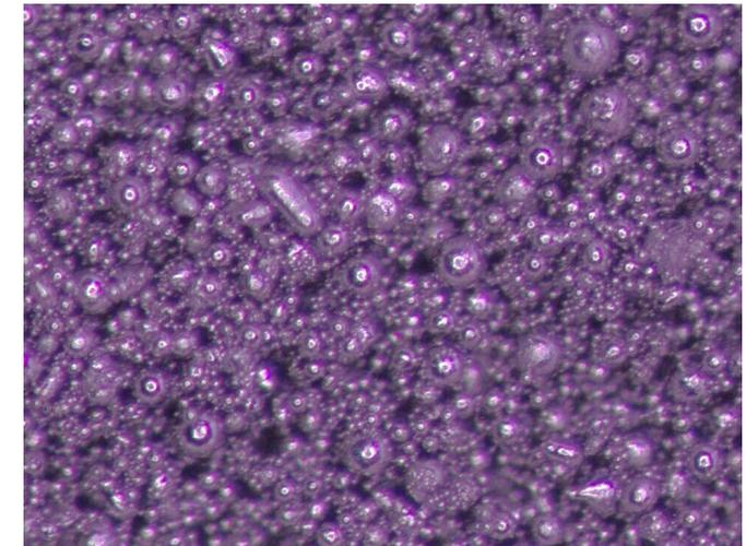
Nickel Alloy Powder in Optical Microscope
