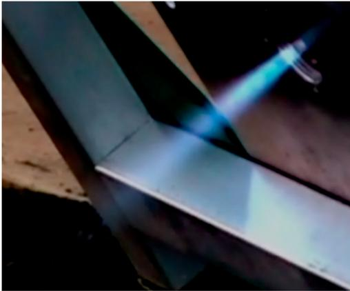
**Figure 11.** Supersonic jet (plume) from LOX/CH<sub>4</sub> thruster showing several faint Mach disks (firing at 2500 m altitude on Mauna Kea).
