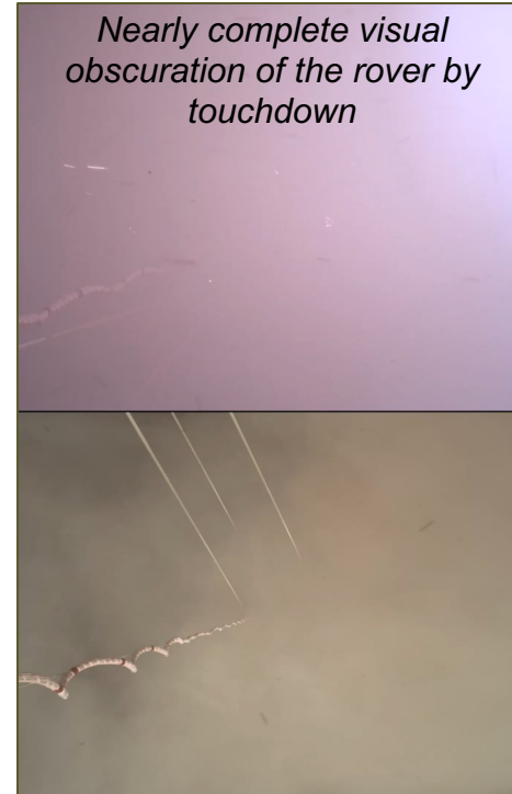
Dust lofting as rover is lowered towards the surface
